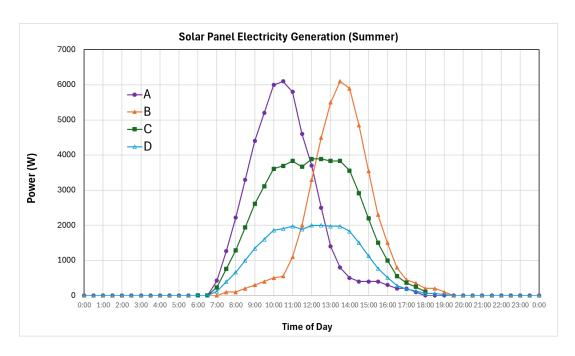
e) In the southern hemisphere the sun moves along the sky much lower to the north than in summer. This changes how much electricity can be generated and has dramatic effects of panels facing different directions. In the solar electricity output diagram below for winter which data represents panels on a roof facing
